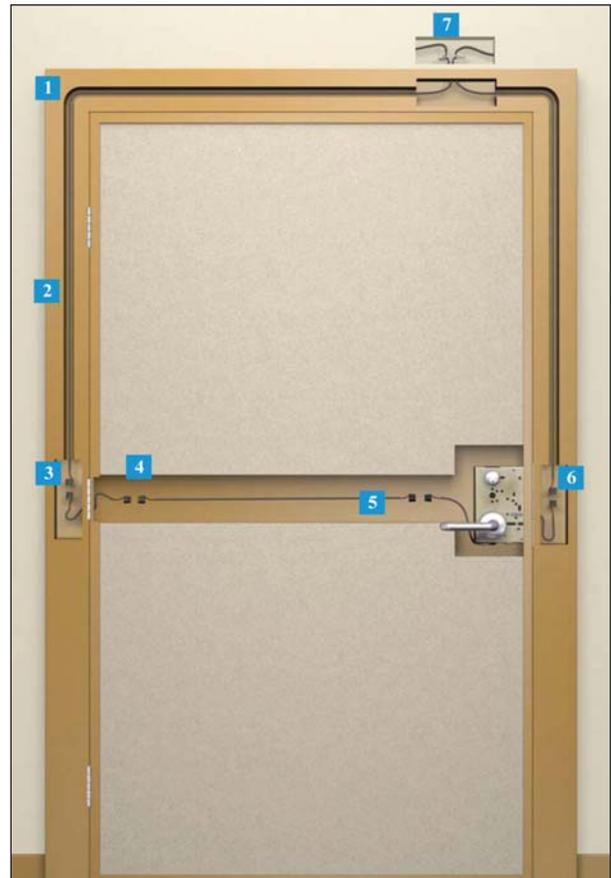
Note: All hardware components utilize a female plug. Doors and frames have a male plug to complete the connection.
