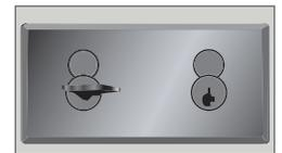
Authorized user key is retained (held captive/trapped) until the high level key is returned to its secure location.
