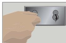
User rotates their release key and now the high level retained key is in the upright position and ready for removal.
