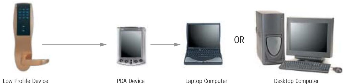
*With the use of a PDA and the SARGENT Soflink Plus w/ Soflink PDP software, transferring data becomes easier and faster. This is an ideal solution for maintaining a large system of access control devices.*
